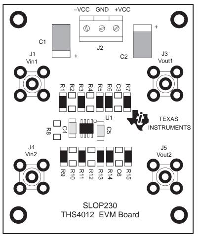
**Note:** The EVM is shipped with the following component locations empty: C3, C6, R2, R4, R8, R10, R12
